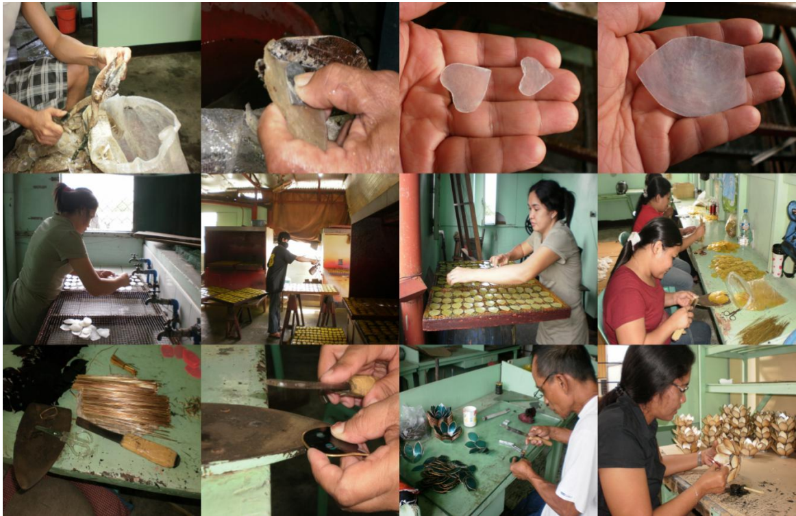
Figure 7.1: In-house capiz production process
